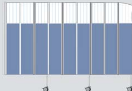
DAYLIGHT TOP Top section is 0.45 m high.
